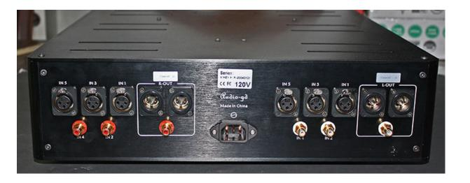
The Audio-gd Vacuum HE1 XLR preamplifier uses fully balanced circuitry from input to the primary (leftmost) XLR output jacks. Balanced circuit design uses two independent amplifiers per channel, one handling the positive swing of the waveform and the other the negative. Most preamplifiers on the market with XLR in and out jacks lack fully balanced circuitry.
